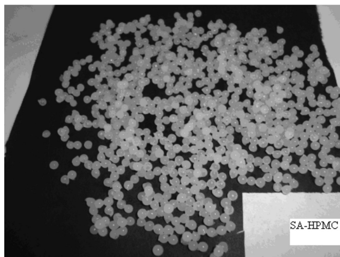
FIGURE 2 - Spherical shape of beads prepared with sodium alginate (SA) and hydrophobic hydroxypropyl methylcellulose (HPMC).
